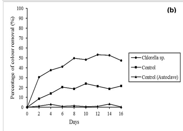
**Figure 5:** The percentage efficiency of (a) COD reduction and (b) colour removal of POME (without dilution) for 16 days.
